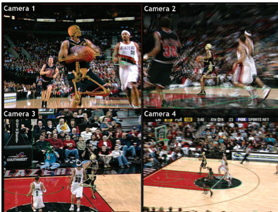
Fig. 1. Matching of the four-camera basketball injury situation 50 ms after initial ground contact. The four panels show the customized skeleton model and the basketball court model superimposed on and matched with the background video image from cameras 1–4. One Poser phantom camera (camera 1) can be seen as a wire-frame model in the bottom left panel as an exact fit.
